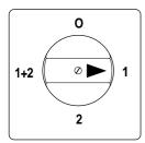
Start pump no. 1 and let the water run from an outlet point of the pipe-line. When connecting a high pressure hose directly to the machine, activate the trigger of the spray handle without the spray lance attached. Let the water run until all air has escaped from the pump (regular water flow).
